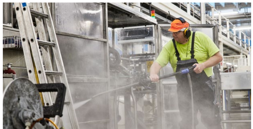
Process water is used for cleaning equipment, floors, surfaces, pipes and tanks, bottle and can washers and more inside the factory.
