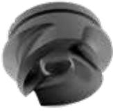
Open **S-tube®** semi-open impellers provide high efficiency over a wide operating range. They can be trimmed to meet a specific duty point, and SE/SL pumps fitted with Open **S-tube®** impellers are the ideal solution for medium to extreme contamination of wastewater.
