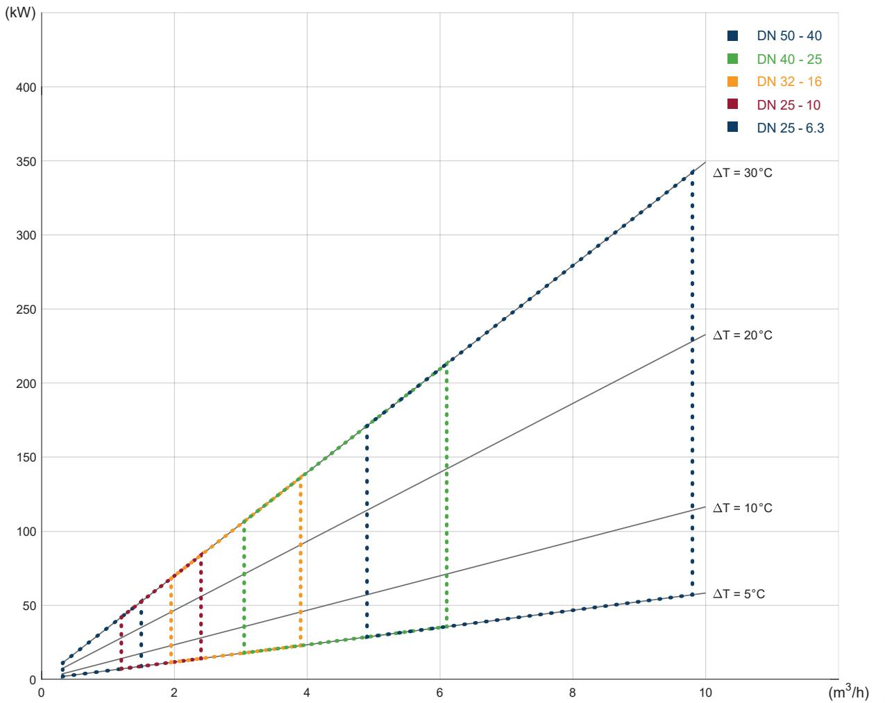
Performance range for three-way MIXIT valve at  $\Delta p_{v100} = 6 \text{ kPa}$
