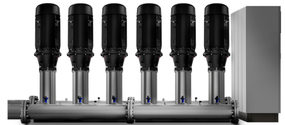
Figure 3: Packaged multipump systems that integrate speed control to quickly ramp throughput up or down can satisfy a broader range of demand with greater energy efficiency than typically offered by end-suction or split-case pumps.
