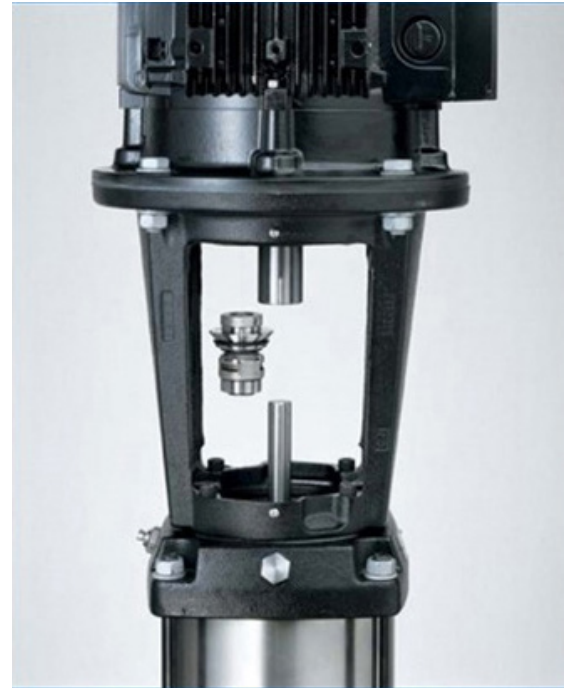
Figure 2: An easily accessible one-piece mechanical shaft seal cartridge can be replaced in minutes, without removing the motor. This avoids the time and effort typically associated with realigning motors and shaft after seal replacement on long-coupled end-suction pumps and split-case pumps.
