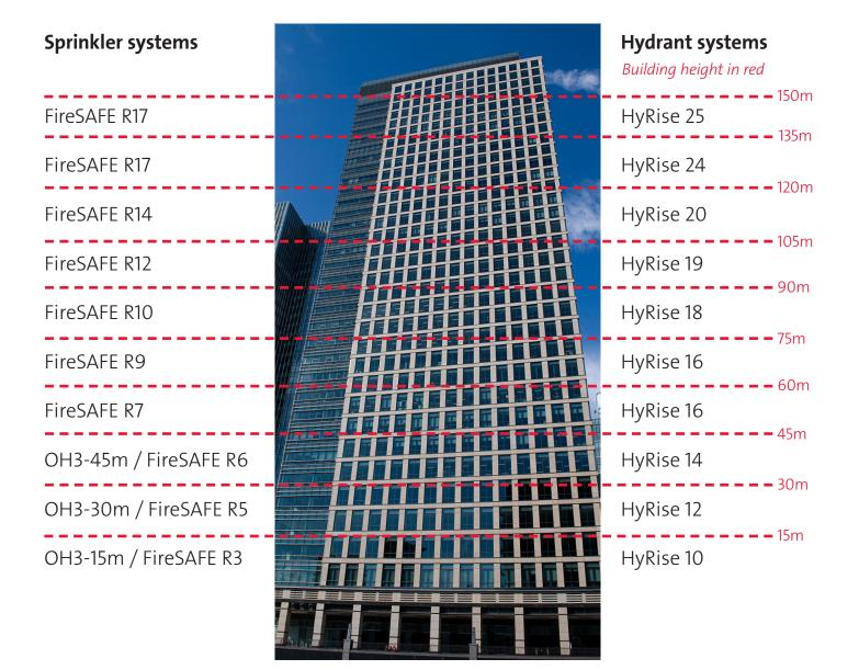
The above image shows a zone indication as to the type of Grundfos sprinkler/hydrant system that may be involved in various high rise fire protection systems. As many other factors will need to be taken into account, any final selection should be ratified by an appropriately qualified design engineer.
