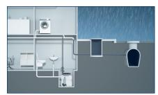
**Lifting station (inside buildings)** Installed in a tank solution in basements and other building spaces below sewer level.
