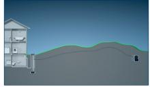
**Pumping station (outside buildings)** Installed outside buildings in a pumping station that leads to a public sewer or a component in pressurised sewage systems in rural areas.
