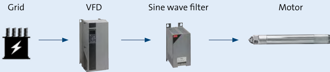
Figure 3: Components of a variable speed motor and pump system. Refer to product manufacturer for proper sizing, voltages, and settings.
